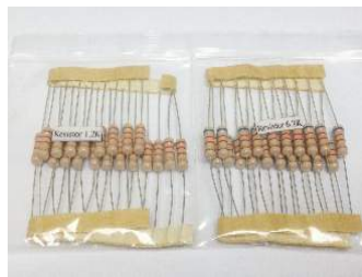
7. Resistors (for tamper detection)
